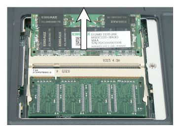
**9** Hold the new or replacement module at a 30-degree angle and press it into the empty memory slot. This module is keyed so it can only be inserted in one direction. If the module does not fit, make sure that the notch in the module lines up with the tab in the memory bay.
