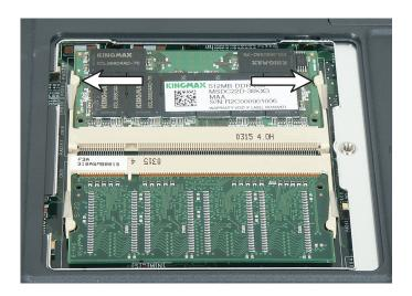
**8** Pull the memory module out of the slot.
